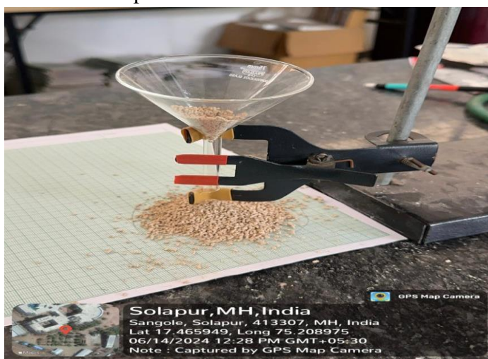
Fig No. 1: Angle of Repose
